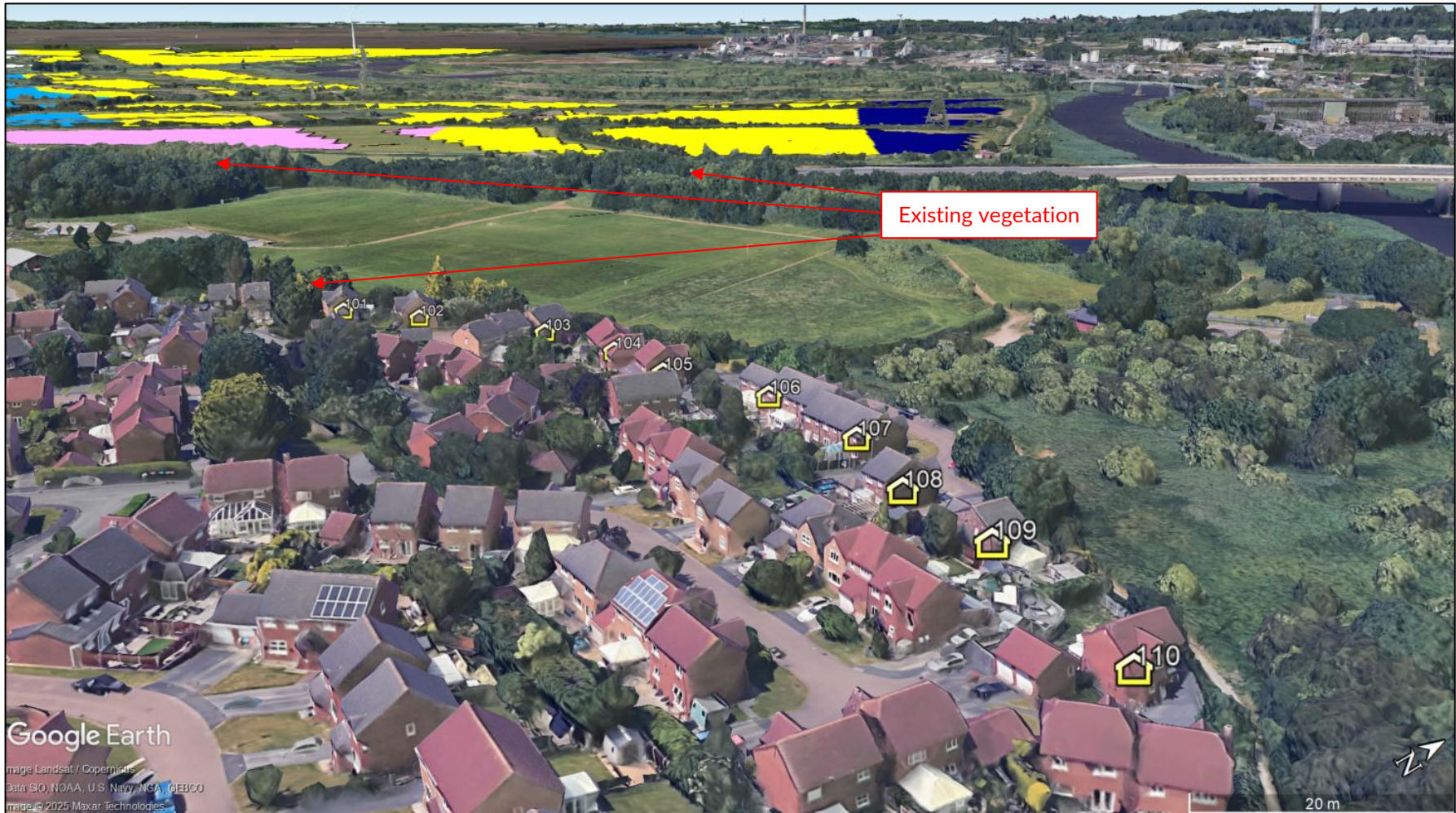
Figure J8583 Reflecting panels and screening for dwelling receptors 101 to 110
