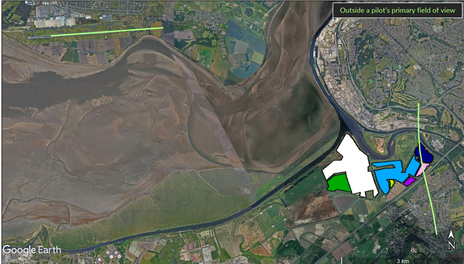
Figure 2019 Solar reflections towards commercial visual approach
