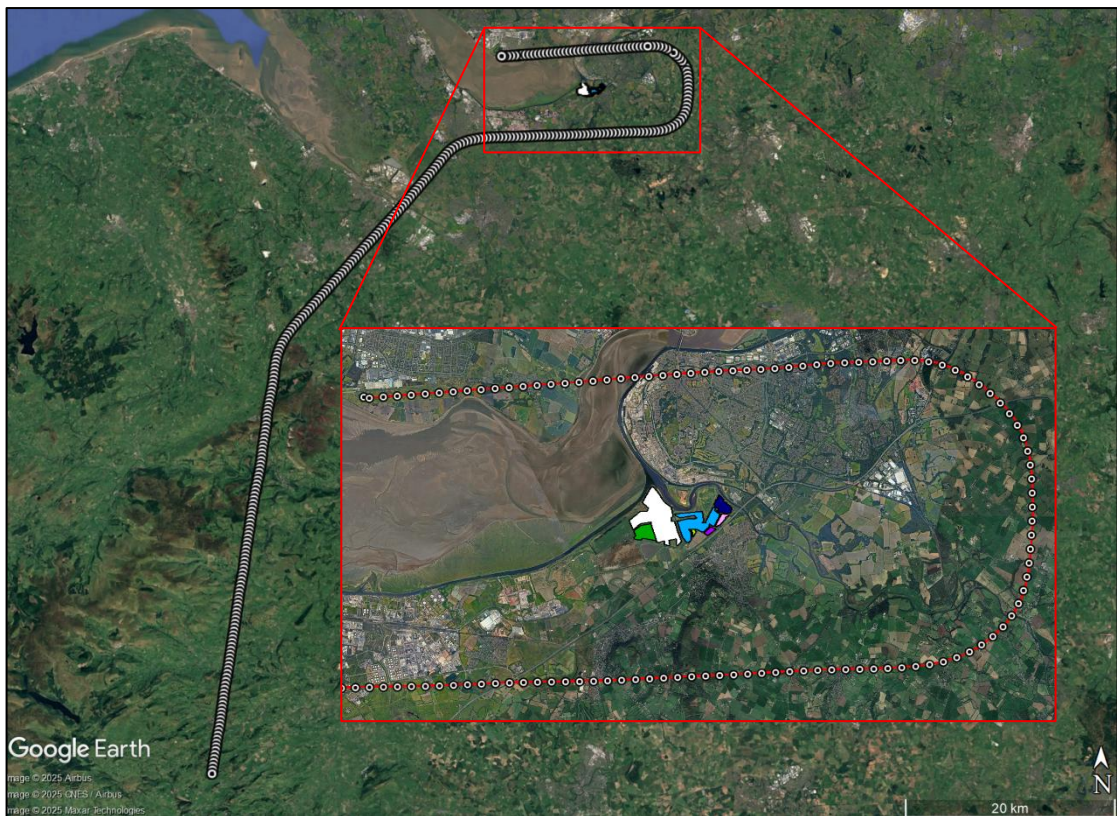
Figure 9 Commercial instrument approach receptors
