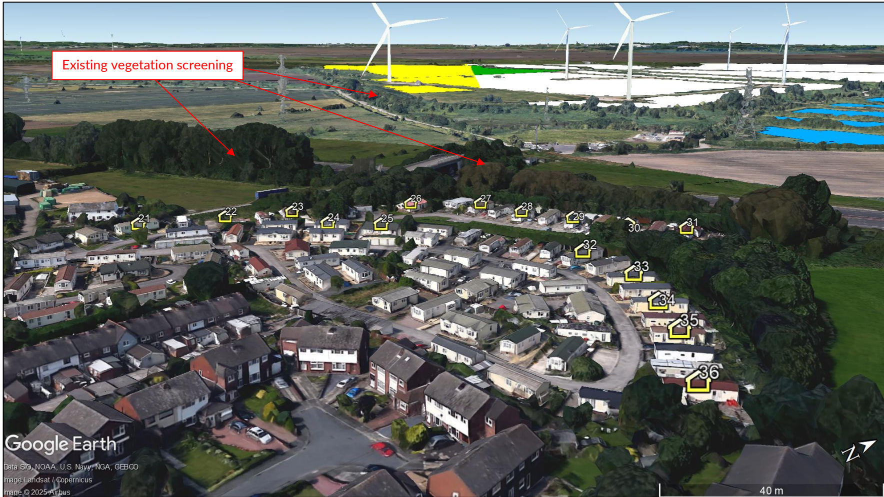
Figure J7472 Reflecting panel areas and screening for dwelling receptors 21 to 36
