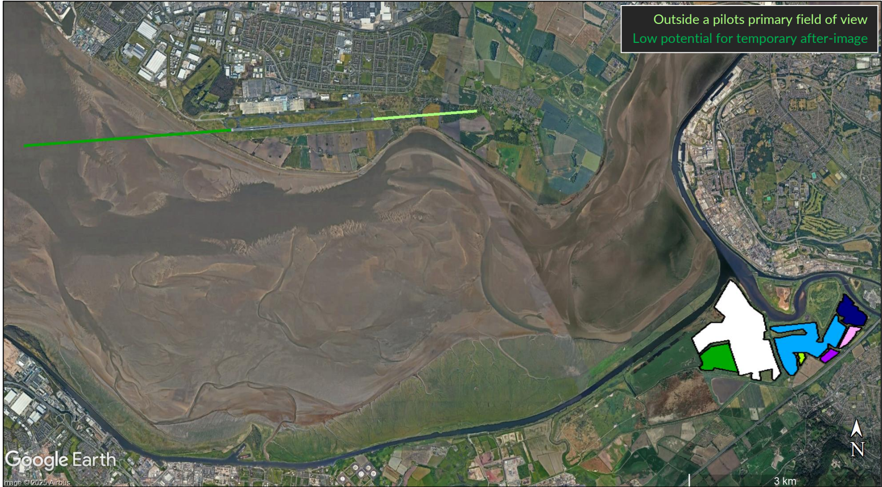
Figure 1716 Solar reflections towards two-mile approaches
