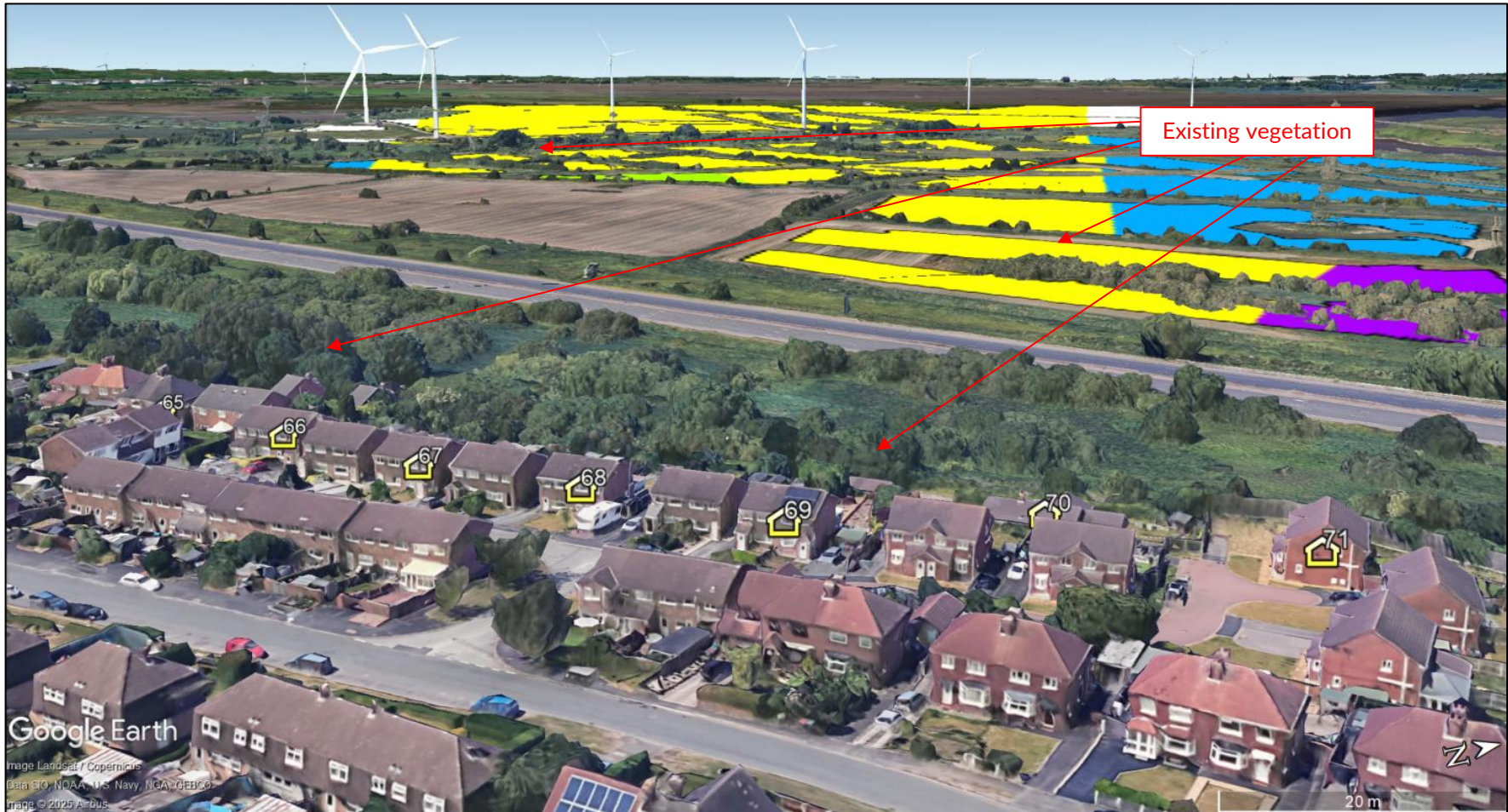
Figure J7876 Reflecting panel area and partial screening for dwelling receptors 65 to 71
