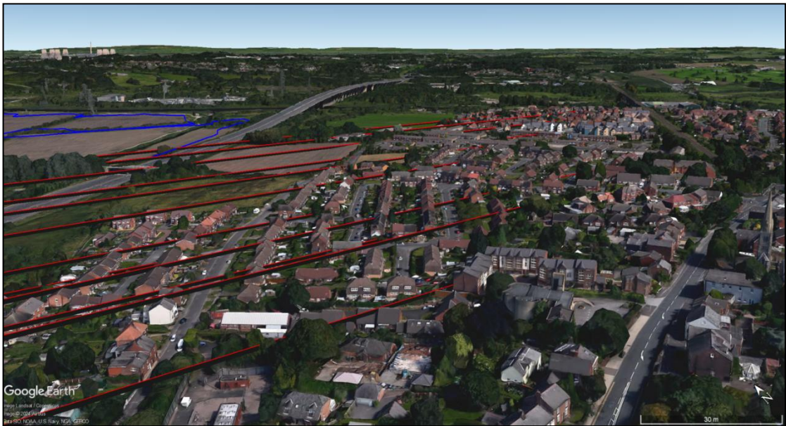
Figure H2826 3D representation of line-of-sight profiles
